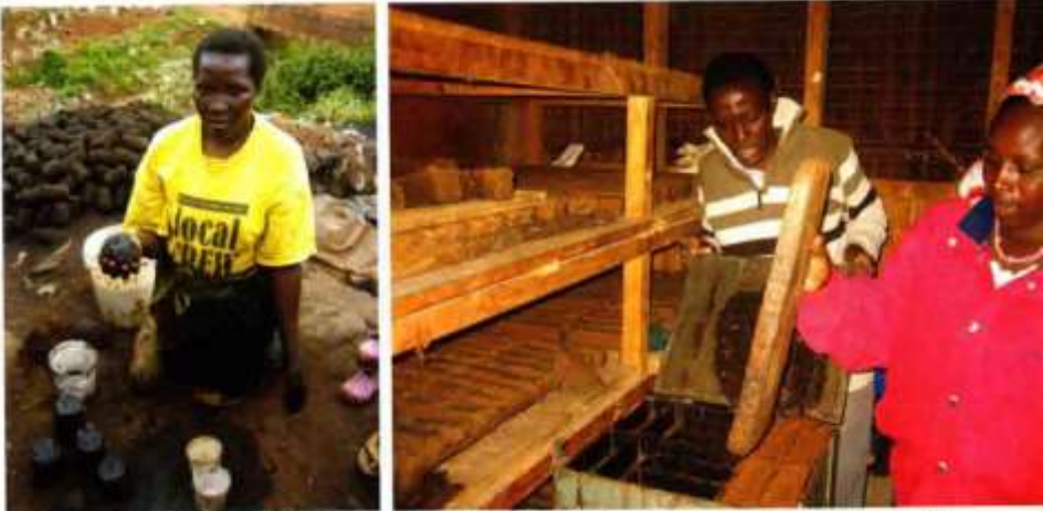
Plate 1: Community based fuel briquettes-making from charcoal dust bound with ash at Kibera (left) and from sawdust bound with gum arabic at Naru Moru (right).
