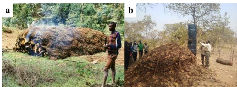
Figure 5: Traditional (a) and improved (b) kilns for charcoal production in Zambia. © FFF, 2019
